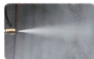
Water-Soluble Minimum Quantity Spray Type Lubricant
